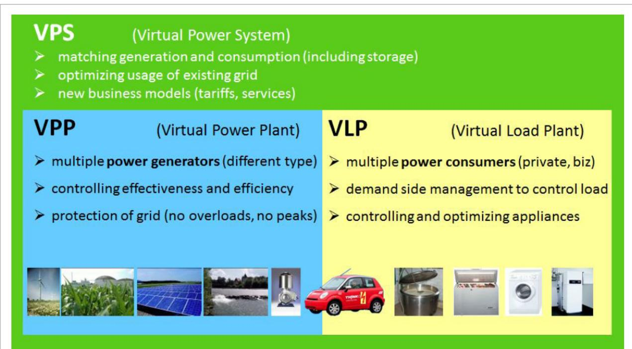
Figure 12 - Concept of a Virtual Power System (Ludwig Karg, 2011)
